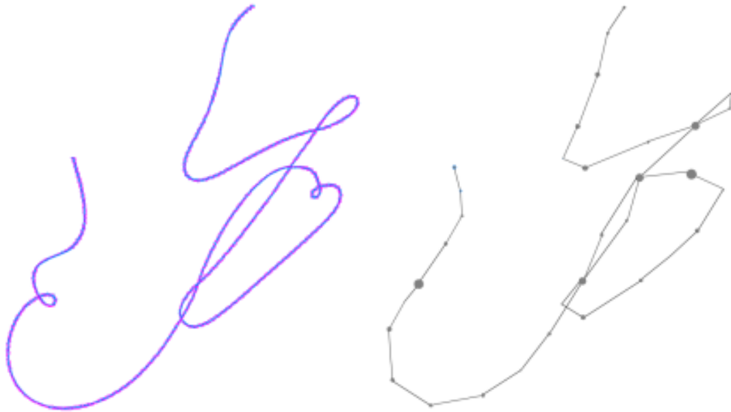
Figure 3.21: On the left a graph drawing of 1000 nodes and 1997 edges. On the right a high level view with 31 nodes and 33 edges.
