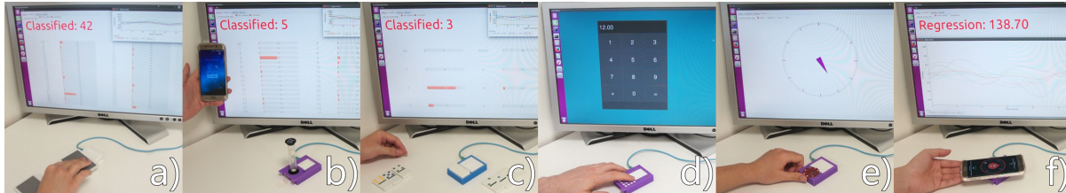
Fig. 6. From left: (a) counting playing cards (b) counting sand in hour glass matched by timer on the smartphone (c) identify Domino pieces (d) identify touch location on a numeric keypad sheet as input for calculator (e) tracking rotation of tagged game piece to control the clock hand and (f) tracking rotation of untagged smartphone using regression.
