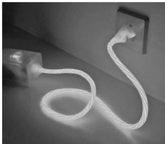
FIGURE 6.11 Power-aware cord, a power-strip designed to actively visualize the energy in use. (Photograph by Magnus Gyllenswård. Accessed from http://tii.se/static/press.htm )
