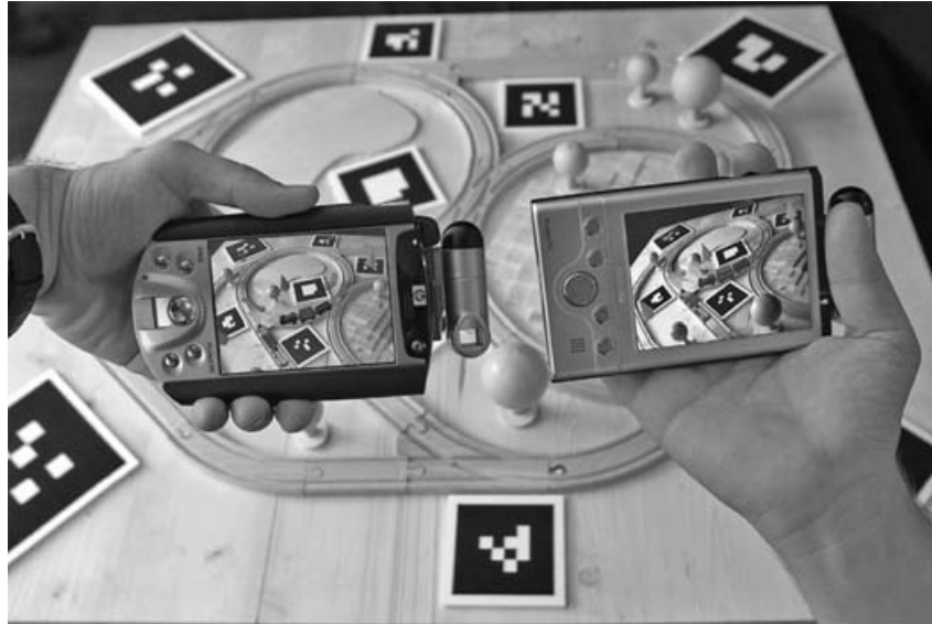
FIGURE 6.5 Augmented Reality invisible train game. (Accessed from Graz University of Technology, http://studierstube.org/handheld_ar/media_press.php )
