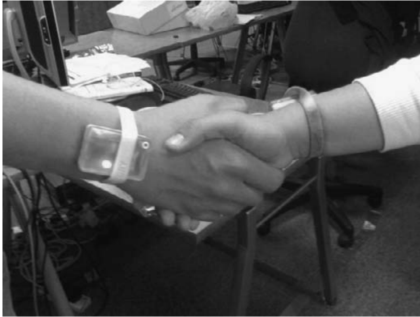
FIGURE 6.15 Matching accelerometer data for sensing handshakes for social network development.
